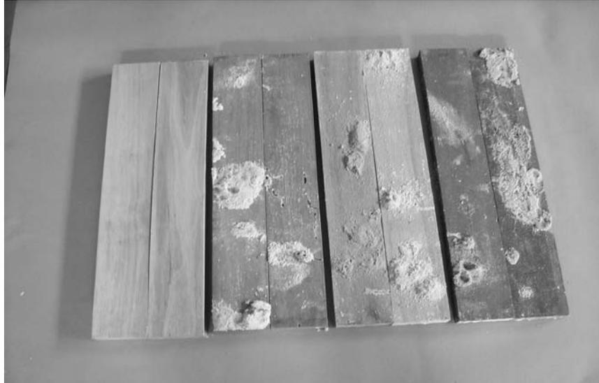
Figure 4. Damage of rubber-wood samples after three years exposure. From left, two samples each, coated with: Melamine, Varnish 1, Varnish 2 and Paint. Samples coated with Melamine were still intact, while others had been badly infested. Frasses shown on wood surface were expelled by larvae or beetles growing inside the samples.
