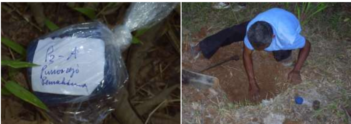
Gambar (Figure) 3. Pengambilan sampel tanah terganggu, dengan plastik; dan tanah tidak terganggu, dengan ring sampel tanah ( Taking of disturbed soil sampling, with plastic; and soil not disturbed, with soil ring samples )
